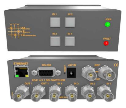
The **MSC-XD41L** SDI routing switcher has 4 inputs and 1 output, supports reclocking of standard 3G/HD/SD SDI rates, automatic bypass of non-standard rates between 20 Mbit/s and 3 Gbit/s, and passes all SDI embedded audio/ancillary data. In addition any output can be independently muted. Switch on vertical sync is provided with the sync reference input with a pass-through connector and provides support for Tri-level sync and NTSC/PAL black burst signals.
